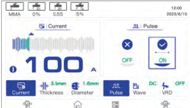
MMA welding interface
